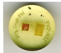
Fig. 1: Resin impregnation followed by surface polishing and ion milling
