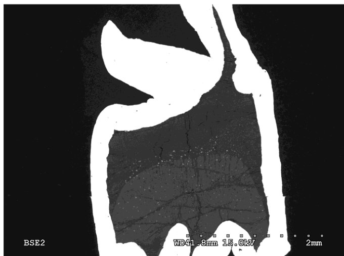
Figure 1: Example of a black shale melting experiment performed at 850°C consisting of approximately 50 % melt (dark area in the top half of the experimental charge).
