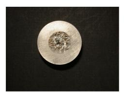
The holder should be transferred to the hot plate set at ~180°C and the indium allowed to melt. Remove and allow to cool.
