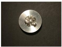
Alternatively, just eye-balling the correct amount of indium works. It maybe advantageous to put less indium in than needed as pressing of the sample can displace enough indium to make the a flat surface across the diameter of the mount.
