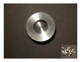
The Al-disk should be cleaned to remove any oils or machining lubricants. The quantity of indium required maybe calculated and then placed in the Al-well. Indium tear-drops can be seen in the bottom right of the picture.
