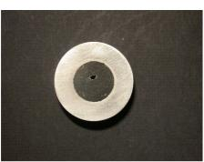
Gently push the sample into the indium and return the holder to the hydraulic press. Again, using the Melinex sheet compress the samples into the indium. The photograph shows a small fragment of a standard pressed into the indium.
