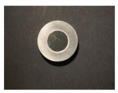
You should now have an aluminum holder with a central well of indium that has a smooth surface. At this stage small troughs can be gouged into the indium to make room for larger samples, so that on pressing the indium does not flow out of the well.
