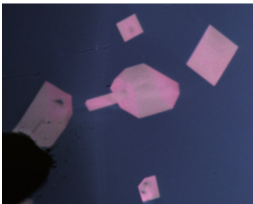
Figure 1: Cathodoluminescence image of synthetic zircon crystals in silicate glass, typical of the samples analysed in this study. The field of view is 500 \mu\text{m} .
